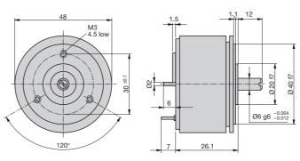
Fig. 9. KINAX 2W2 with special drive shaft at front **and** at rear. At front: Ø 6 mm, length 12 mm. At rear: Ø 2 mm, length 6 mm.
