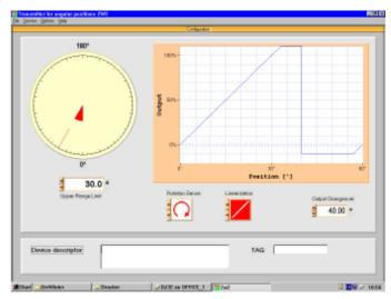
Fig. 4. Print screen example of the menu-controlled programming software.
