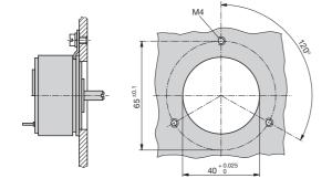
Fig. 12. Drilling plan for fixing with 3 spring clamps.
