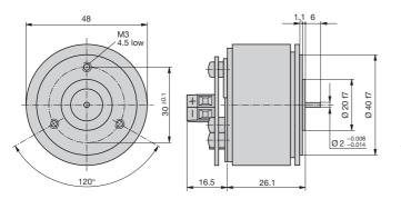
Fig. 6. KINAX 2W2 with standard drive shaft at front **only**, Ø 2 mm, length 6 mm, screw terminal version.
