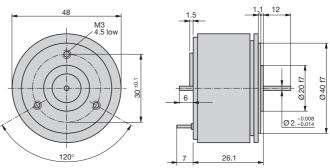
Fig. 7. KINAX 2W2 with special shaft drive at front **and** at rear. At front: Ø 2 mm, length 12 mm. At rear: Ø 2 mm, length 6 mm.
