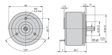
Fig. 8. KINAX 2W2 with special drive shaft at front **only**,  $\emptyset$  6 mm, length 12 mm.
