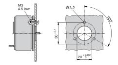
Fig. 13. Drilling plan for fixing with 3 cheesehead screws M3.
